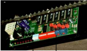
Panic and Worklight switches
