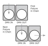
2. Connect the end of the cable coming from the first fixture which will have a female connector to the input connector of the next fixture consisting of a male connector. Then, proceed to connect from the output as stated above to the input of the following fixture and so on.
