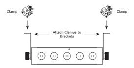
Mount the fixture using a suitable "C" or "O" type clamp. The clamps should be rated to hold at least 10x the fixture's weight to ensure structural stability. Do not mount to surfaces of unknown strength, and ensure properly rated rigging is used when mounting fixtures overhead.
