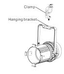
**NOTE:** Various types of truss hooks can be used. The hook (as shown in the example above) as well as many other standard hooks, can be ordered separately.
