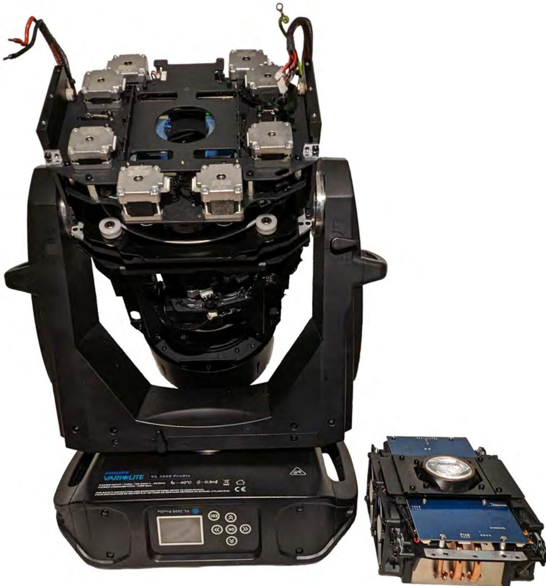
**Repeat the process in reverse installing your new Upgraded LED Assembly**
