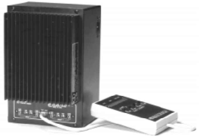
Dual 10A Automatic Dimmer with hand-held test unit
