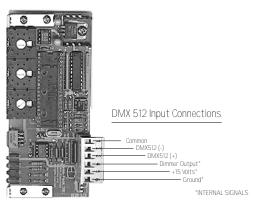
All wiring must be rated for at least 150VAC
